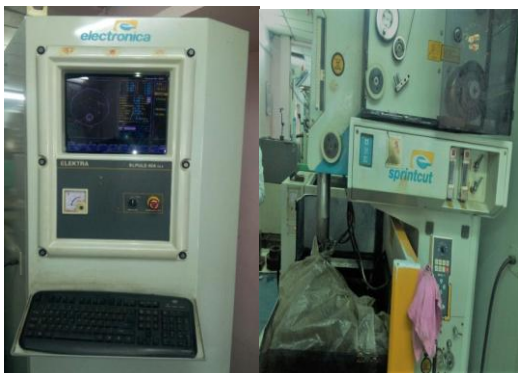
Fig 1: Electronica –Elektra-Elpuls 40 a DLX wire EDM
